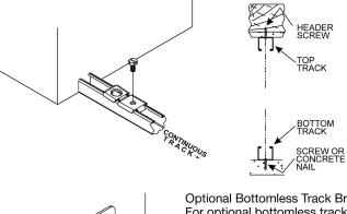
Optional Bottomless Track Bracket -For optional bottomless track bracket, set bracket on floor directly below top track. Fasten bracket to the wall
